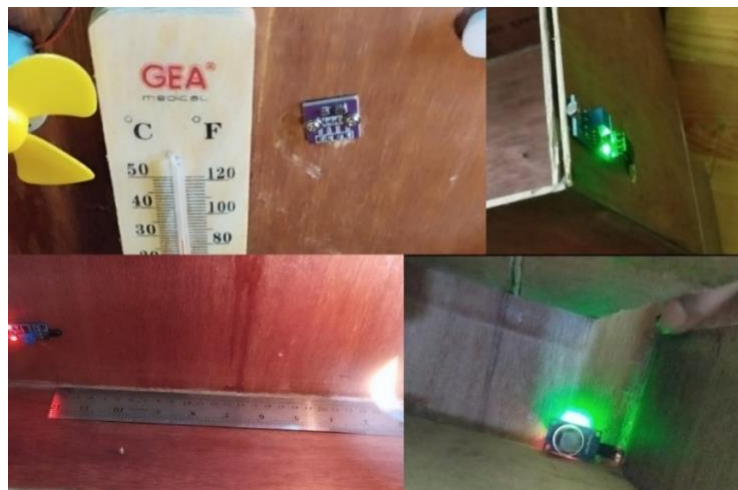
Fig. 5: Experimental setup for evaluating the AHT20, MQ-2, flame, and LDR sensors
