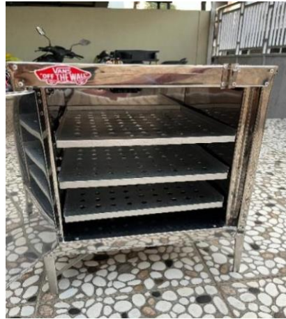
Fig. 4: Final prototype of the automatic rengginang dryer (interior)
