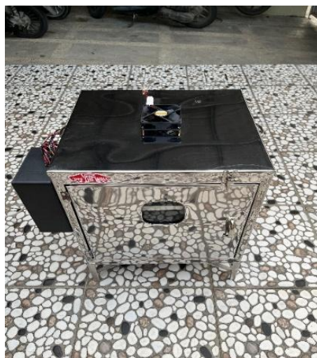
Fig. 3: Final prototype of the automatic rengginang dryer (exterior)
