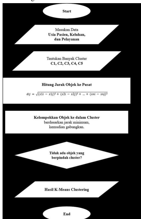
Fig. 1: K-means clustering procedure used in the study
