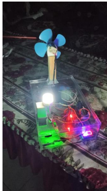
Fig. 7: Automatic lamp test under dark conditions
