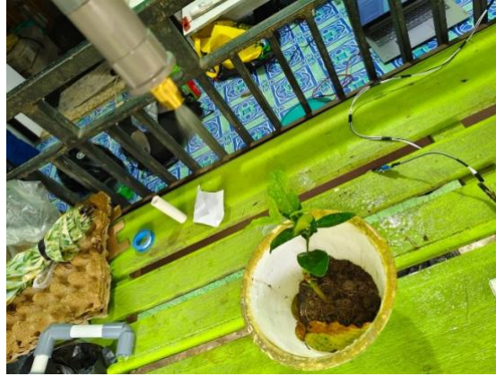
Fig 11: System Activating Pump under Dry Conditions
