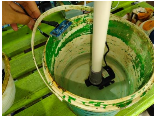
Fig 12: Buzzer Alert when Water Level is Below 20%
