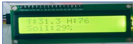
Fig. 5: I2C LCD interface
