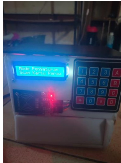
Fig. 5: LCD Display Upon Entering Configuration Mode
